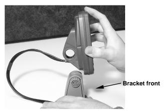
Mount the sonar: slide the unit onto the bracket from above.
